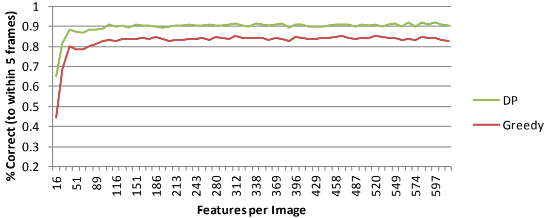
Figure 2.17: Accuracy increases with the number of features per image. Images corrupted with noise of \sigma = 32 .
